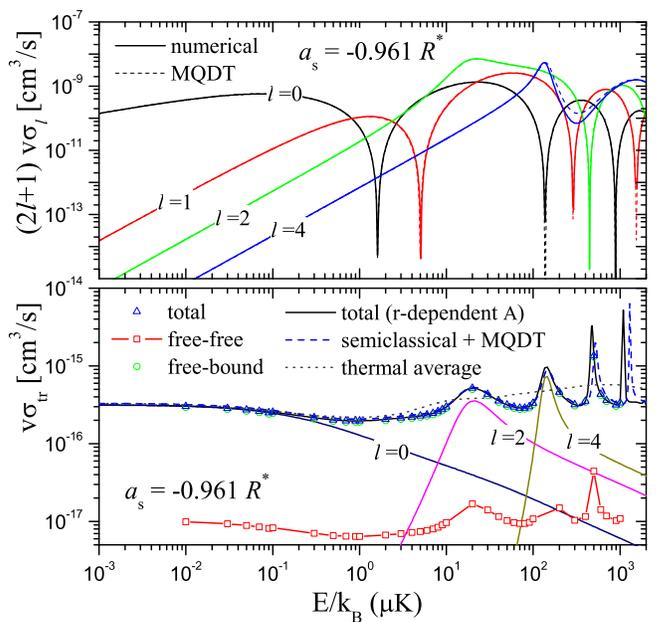
FIG. 1: Elastic collision rate in the singlet channel  $A^1\Sigma^+$  (upper panel) and rate of radiative  $A^1\Sigma^+ \rightarrow X^1\Sigma^+$  charge transfer (lower panel) versus collision energy. Different theoretical approaches are compared (see text). Both the elastic and the total inelastic rate are decomposed on selected partial waves.
