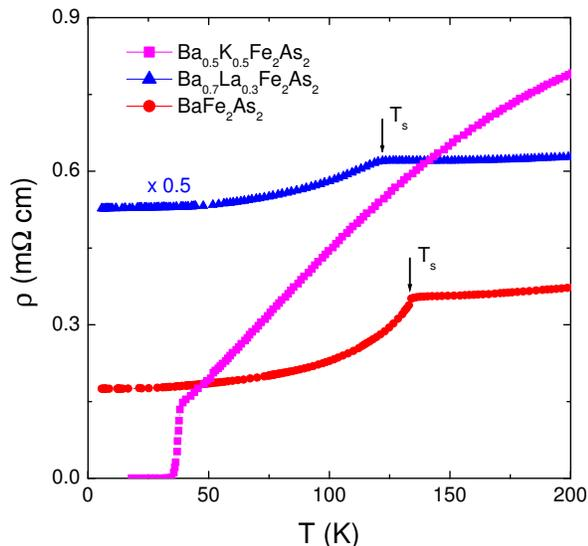
FIG. 1: (Color online) Resistivity of  $\text{BaFe}_2\text{As}_2$  single crystal, electron-doped  $\text{Ba}_{0.7}\text{La}_{0.3}\text{Fe}_2\text{As}_2$  and hole-doped  $\text{Ba}_{0.5}\text{K}_{0.5}\text{Fe}_2\text{As}_2$  polycrystals. Arrows denote the structural and antiferromagnetic transitions occurring at the same temperature  $T_s$ .
