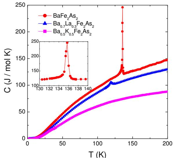
FIG. 2: (Color online) Specific heat of  $\text{BaFe}_2\text{As}_2$ ,  $\text{Ba}_{0.7}\text{La}_{0.3}\text{Fe}_2\text{As}_2$  and  $\text{Ba}_{0.5}\text{K}_{0.5}\text{Fe}_2\text{As}_2$  samples. The parent compound  $\text{BaFe}_2\text{As}_2$  single crystal shows a very sharp peak at 136 K, enlarged in the insert. A small peak is also visible at 120 K for  $\text{Ba}_{0.7}\text{La}_{0.3}\text{Fe}_2\text{As}_2$ .
