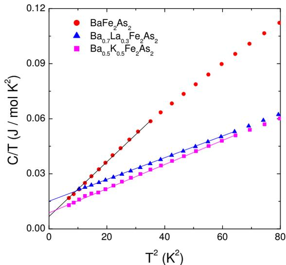
FIG. 4: (Color online)  $C/T$  vs  $T^2$  for  $\text{BaFe}_2\text{As}_2$ ,  $\text{Ba}_{0.7}\text{La}_{0.3}\text{Fe}_2\text{As}_2$  and  $\text{Ba}_{0.5}\text{K}_{0.5}\text{Fe}_2\text{As}_2$  samples. The lines are linear fits at low temperature.
