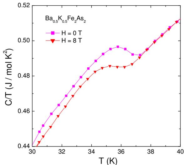
FIG. 3: (Color online)  $C/T$  vs  $T$  for  $\text{Ba}_{0.5}\text{K}_{0.5}\text{Fe}_2\text{As}_2$  polycrystalline sample near  $T_c = 36$  K in zero and  $H = 8$  T magnetic fields. Rough estimation gives the specific heat jump  $\Delta C/T \approx 15$  mJ / mol  $\text{K}^2$  at  $T_c$  in zero field.
