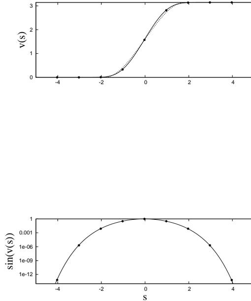
FIG. 7: Top panel: The wave form of the compact kink solution between  $v^* = 0$  and  $\bar{v}^* = \pi$  for the coupling  $q(v) = \cos v$ . Markers show the wave form on the discrete lattice and the dashed line represents the quasi-continuum approximation of the kink. Bottom panel: The sine of the kink in logarithmic scale.
