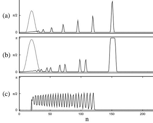
FIG. 11: Evolution of different initial pulses for the coupling  $q(v) = \cos v$  and  $v^* = 0$ . The initial conditions were set according to (32). (a)  $w = 10$  and  $A = 2$ , (b)  $w = 15$  and  $A = 3$  and (c)  $w = 1$  and  $A = 1$ . The dashed line shows the initial condition  $v_n(t = 0)$  and the solid line the lattice at the time  $t = 100$ .
