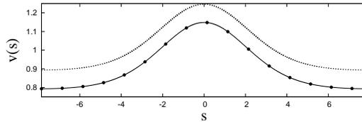
FIG. 9: The shape of a periodic wave on the lattice. The offset is  $v^* = \pi/4$ , the wave length is  $w = 5\pi$  and the velocity  $\lambda = \pi/2$ .
