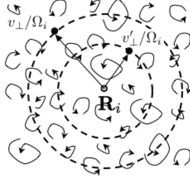
Figure 1. The nonlinear perpendicular phase mixing: the gyrocentre distribution function at a given point \mathbf{R}_i is mixed in a decorrelated way by \mathbf{E} \times \mathbf{B} flows gyroaveraged over ion orbits whose radii ( v_{\perp}/\Omega_i and v'_{\perp}/\Omega_i ) differ by more than the flows' correlation length.
