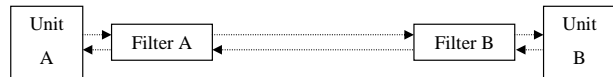
FIG. 2: A setup of two time-delayed mutually coupled units, where each unit has a filter influencing both transmitted and received signals.
