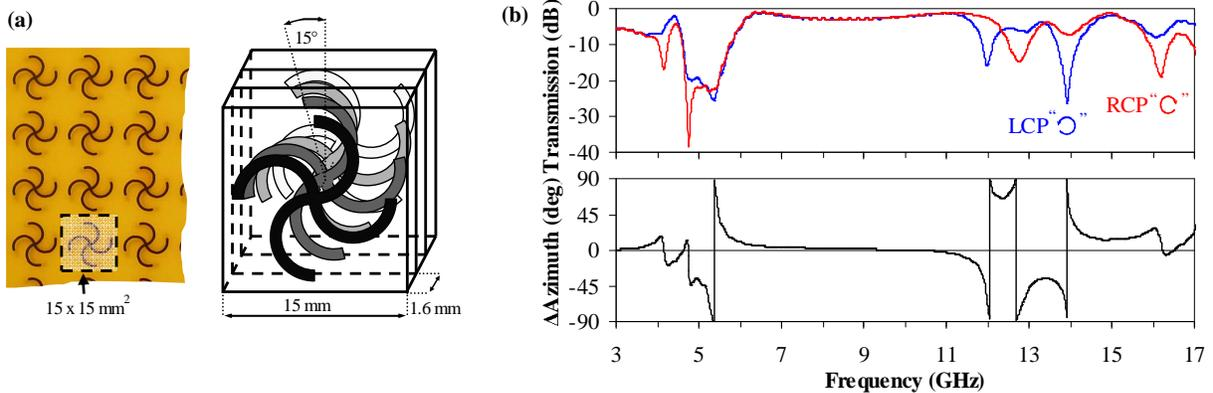
FIG. 2: The 4-layered version of the metamaterial. (a) A fragment of the 4-layered material and schematics of its three-dimensionally chiral unit cell. (b) Transmission levels for right-handed (RCP) and left-handed (LCP) circular polarizations and azimuth rotation for linear polarization.
