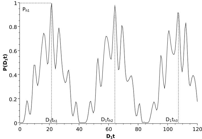
Fig. 2. Probability of the state transfer along the six-nodes spin chain with  $\delta_{h_1} = 2.373$ ;  $P_{h_1} = 0.997$  is achieved at  $D_1 t_{h_1} = 21.428$ .
