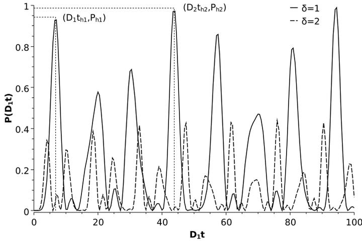
Fig. 6. Comparison of probabilities for the state transfer along the two five-spin chains with  $\delta = 1$  ( $\lambda_1 = 1.732D_1$ ,  $\lambda_2 = D_1$ ) and  $\delta = 2$  ( $\lambda_1 = 2.646D_1$ ,  $\lambda_2 = 1.732D_1$ )
