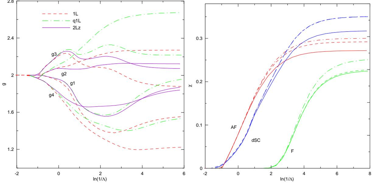
FIG. 7: (color online) The flow of the vertices (a) and the susceptibilities (b) of the 2D  $t$ - $t'$  Hubbard model,  $U = 2t$ ,  $t'/t = 0.1$ ,  $\mu = -0.5t$ , and  $T = 0.025t$  in the 24-patch one- and two-loop fRG approaches, the notations are the same as in Fig. 6.
