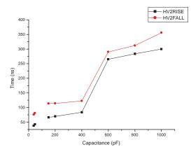
Figure 9. HV2 rise and fall time measurements versus capacitive load.
