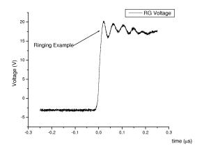
Figure 7. RG Ringing Output Voltage for a 51pF load.
