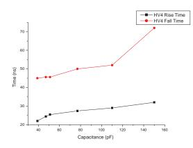
Figure 11. HV4 rise and fall time measurements versus capacitive load.
