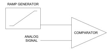
Figure 13. General architecture for the ADC Comparator structure.
