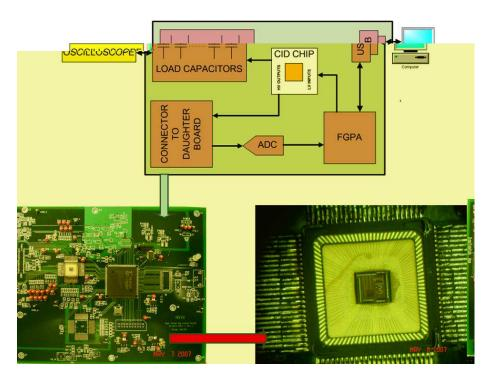
**Figure 4.** Top image shows the general schematic of the system developed to use the High Voltage Chip, the connector to the daughter board correspond to the CCD connector. The bottom left image shows a photograph of the real board, where the chip can be observed on the left top side of the image. The bottom right image shows a photograph of the chip, where all the wire bondings done (with lengths of  $\sim$ 3mm have been used) can be observed.
