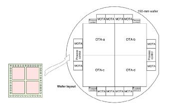
Figure 1. Basic Mini-OTA locations on wafer.
