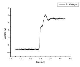
Figure 6. S1 Output voltage signal for a 300pF load capacitance.
