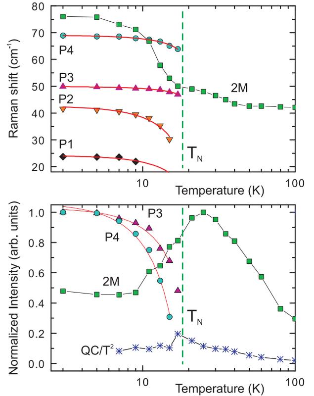
FIG. 5: (Online color) (Upper panel) Peak frequency of the magnetic signals, Pi ( $i=1-4$ ) and the two-magnon continuum, 2M for  $\text{Cu}_2\text{Te}_2\text{O}_5\text{Cl}_2$  on a logarithmic temperature scale. (Lower panel) Scattering intensity of the magnetic signals. The intensity of quasielastic scattering, QC, is normalized by  $T^2$  to be compared with the magnetic specific heat.<sup>8</sup> Lines are guides to the eye.
