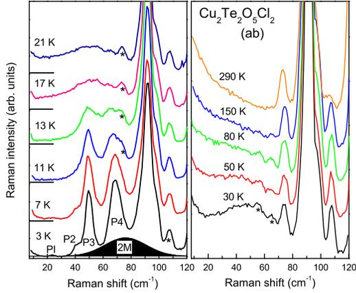
FIG. 4: (Online color) Temperature dependence of low-frequency Raman spectra in (ab) polarization. The asterisks denote low-frequency phonon modes. Pi ( $i=1-4$ ) and 2M correspond to the four sharp magnetic signals and the two-magnon continuum, respectively.
