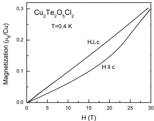
FIG. 2: High-field magnetization of  $\text{Cu}_2\text{Te}_2\text{O}_5\text{Cl}_2$  for  $H \parallel c$  and  $H \perp c$  axis at  $T=0.4$  K, respectively, measured using a pulsed magnetic field.
