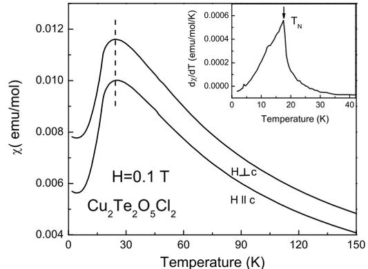
FIG. 1: Temperature dependence of magnetic susceptibility of  $\text{Cu}_2\text{Te}_2\text{O}_5\text{Cl}_2$ ,  $\chi(T)$ , in an applied field of  $H = 0.1$  T for  $H \parallel c$  and  $H \perp c$  axis, respectively. Inset: derivative of magnetic susceptibility,  $d\chi/dT$ . The kink at  $T_N^{\text{Cl}} = 18.2$  K corresponds to long-range magnetic ordering.
