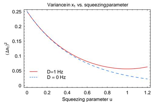
FIG. 2: Variance in the quadrature component  $x_1$  (Eq. 12), vs. squeezing parameter  $u$ , for a SrO molecule interacting with a cantilever. The two curves are for the cantilever damping rates linewidth  $D = 1$  Hz (solid curve) and  $0$  Hz (dashed curve). Squeezing occurs when the variance in  $x_1$  is below  $1/4$ , and is eventually destroyed due to phase noise in the cantilever.
