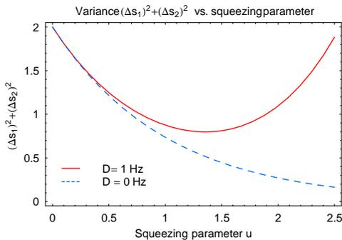
FIG. 3: Sum of variances of  $s_1$  and  $s_2$ , vs. squeezing parameter  $u$ , for a SrO dipolar crystal interacting with a cantilever. The two curves are for cantilever damping rates of  $D = 1$  Hz (solid curve) and  $0$  Hz (dashed curve). Phase fluctuations of the cantilever eventually increase the sum of variances to a value larger than 2, indicative of the loss of entanglement between the two phonon modes.
