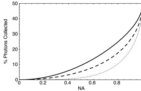
Fig. 4. Fraction of light captured as a function of lens NA. Solid black line (upper) is for a  $\pi$  transition oriented along equator (optical axis perpendicular to magnetic field) and  $\sigma$  transitions oriented along the pole (optical axis parallel with magnetic field). Dashed line (middle) is  $\sigma$  light from equatorial orientation, Dotted line (lower) is  $\pi$  transition light from polar orientation.
