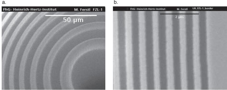
Fig. 2. Electron microscopy images of the patterned phase Fresnel lens surface. a. Center region showing the innermost rings. b. Edge region with structures of comparable size to the  $\lambda = 369.5$  nm design wavelength. Images courtesy of M. Ferstl, Heinrich-Hertz-Institut of the Fraunhofer-Institut für Nachrichtentechnik.
