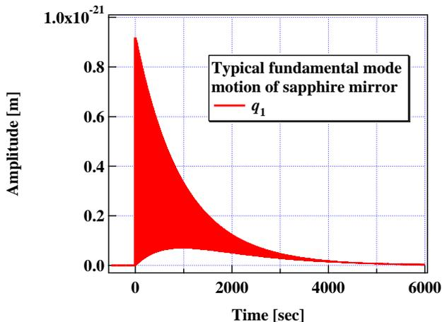
FIG. 2: Vibration of the fundamental mode caused by a low-energy cosmic-ray muon in the time domain,  $q_1$  in Eq. (35). In the calculation, the material values of sapphire at room temperature are used. Since the Q-value is extremely high, i.e. the decay time is longer than the period of the resonant motion, we are not able to see the resonant motion of the one period in this graph.
