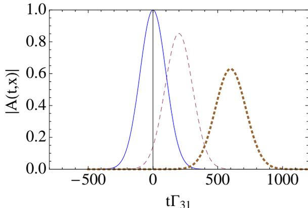
FIG. 5: (Color online) The pulse propagation profile as a function of time,  $t\Gamma_{31}$ , at different locations near the interface: blue (solid) at  $x = 0$ , red (dashed) at  $x_1 = 1\text{mm}$ , and brown (dotted) at  $x_2 = 3\text{mm}$ .
