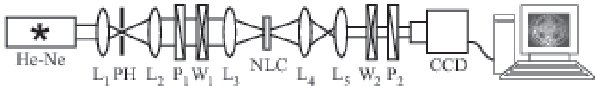
FIG. 1: Experimental setup: He-Ne is the laser; L_1 , L_2 and L_5 are the collimating lenses; L_3 and L_4 are the microscope objectives; PH is the pinhole; NLC is the NLC cell; P_1 and P_2 are the polarizers; W_1 and W_2 are the quarter wave plates; CCD is the CCD camera. A microscope objective L_3 is illuminated with an elliptically polarized and expanded parallel beam of light from a He-Ne laser. The output from a second objective L_4 is collected by a CCD camera through the Stokes analyzer.
