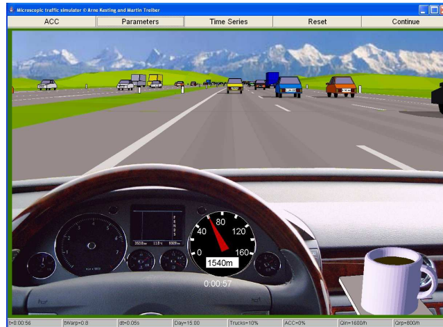
Figure 11: Example of a 3D animation from the driver perspective. Notice that the “Coffeemeter” visualizes the acceleration and the jerk (the changes of all acceleration with time) which are difficult to visualize by other means. It therefore serves as a measure of the driving comfort.
