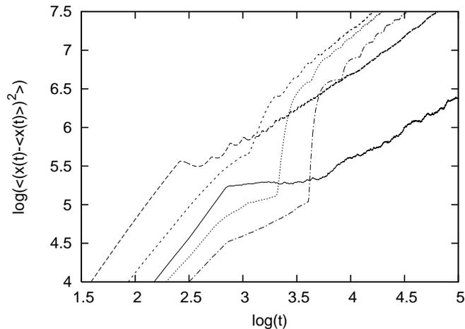
FIG. 7: The position dispersions  $\langle (\Delta x)^2 \rangle$  as a function of time  $t$  are shown for the square wave drive amplitude  $F_0 = 0.2$  but with periods 500 (long dashed line), 2000 (small dashed line), 4000 (dotted line), and 8000 (dashed-dotted line) for  $\gamma = 0.035$ ,  $T = 0.4$ , and  $\phi = 0.35$ . The dispersions when a constant force  $F_0 = 0.2$  is applied is shown by the solid line. This curve is analogous to the homogeneous case of [7].
