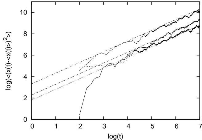
FIG. 6: The position dispersions  $\langle (\Delta x)^2 \rangle$  are plotted as a function of time  $t$  for  $F_0 = 0.08$  (solid line), 0.3 (dashed line) and 0.6 (small dashed line) for  $\gamma = 0.035$  and  $T = 0.4$ . The straight lines are drawn to indicate the average slope equal to 1 and intercepts 1.8, 3.2 and 2.27 respectively for the above  $F_0$  values of the curves at large  $t$  limit.
