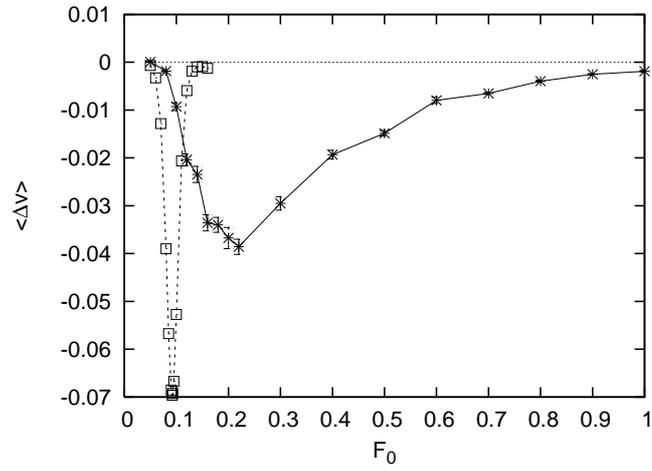
FIG. 5: The ratchet current  $\langle \Delta v \rangle$  when the system was driven by a square-wave field of amplitude  $F_0$  are shown (+) with errorbars for  $\gamma_0 = 0.035$  and  $T = 0.4$ . The curve (with open box) is for the adiabatic case for the same  $\gamma_0$  and  $T$
