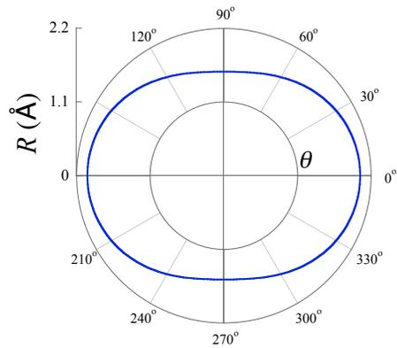
Fig. 3. Equipotential line  $R(\theta)$  for the  $\text{Na}^+ - \text{N}_2$  potential energy surface at a collision energy of 5 eV. The Legendre moments, Eq. (7), of the potential energy surface are listed in Table 1.
