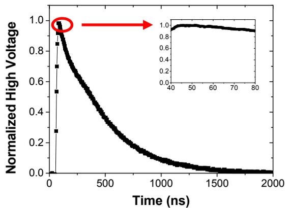
FIG. 3: Trend of the high voltage signal as function of time. Inset: the trigger signal remain constant for almost  $10ns$ .
