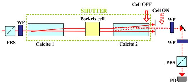
FIG. 4: Experimental setup. A PBS and a  $\lambda/2$  waveplate allow to vary the polarization of the input beam **a**. A second PBS and  $\lambda/2$  waveplate analyze the polarization state of the output beam **b**. The signal is detected by a photodiode (PD).
