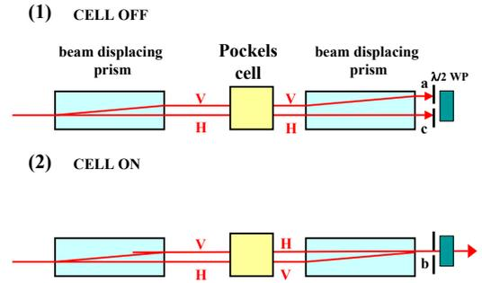
FIG. 1: Experimental scheme of the shutter: (1) when the shutter is off the two beams separated by the two calcites are stopped by the pin-hole (modes **a** and **c**). (2) On the contrary when the shutter is on the two beams are recombined on the second calcite and the resulting beam (mode **b**) passes through the pin-hole.
