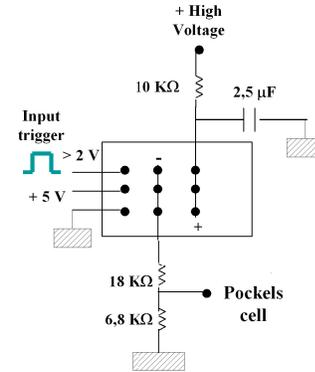
FIG. 2: Electronic driver of the Pockels cell. When the signal of the trigger is on the PC is activated.
