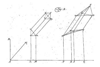
**23**. Whatever the later motion of the point  $\lambda$ , it can be resolved following the three directions  $\lambda \mu$ ,  $\lambda \nu$ ,  $\lambda o$ , parallel to the axes *AL*, *AB* and *AC*. For the motion of the point  $\lambda$  we set
