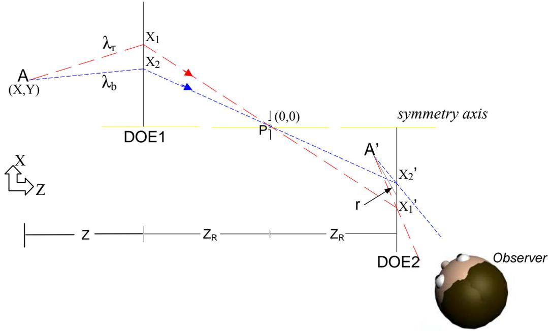
Figure 3. Ray-tracing for the image of a point white-light object.
