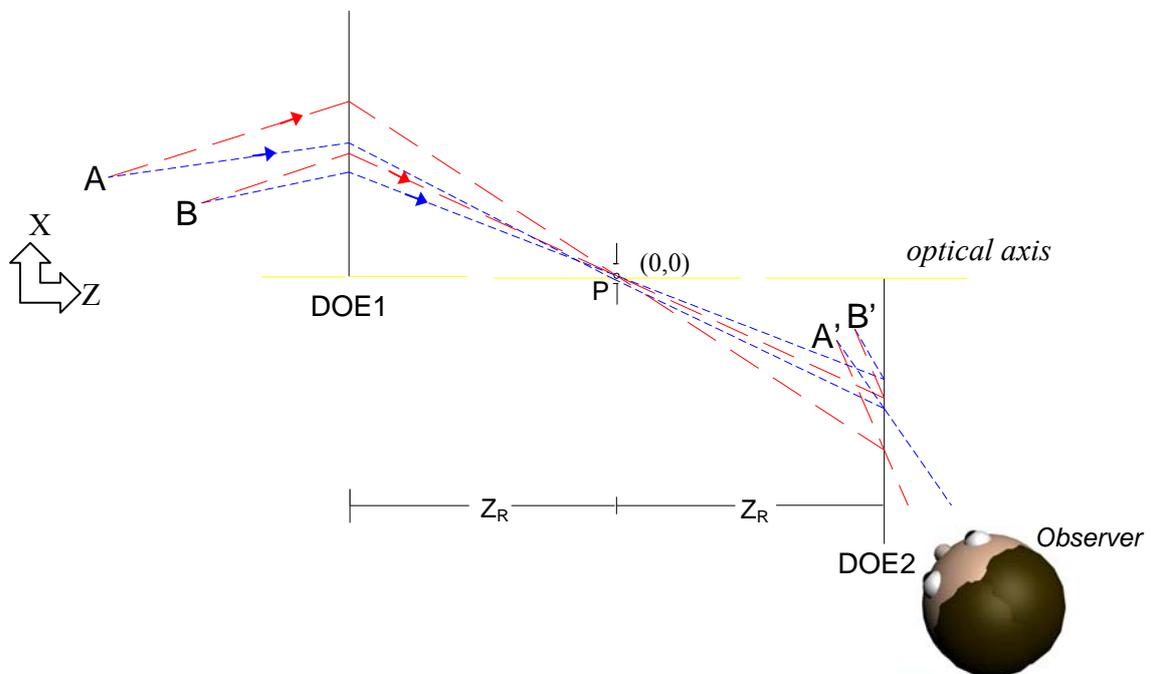
Figure 4. Ray-tracing scheme for the normal depth image.
