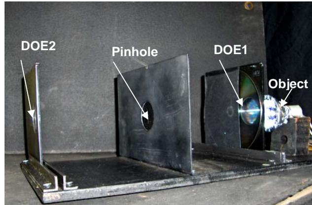
Figure 6. Experimental setup of a double diffraction system with a pinhole.
