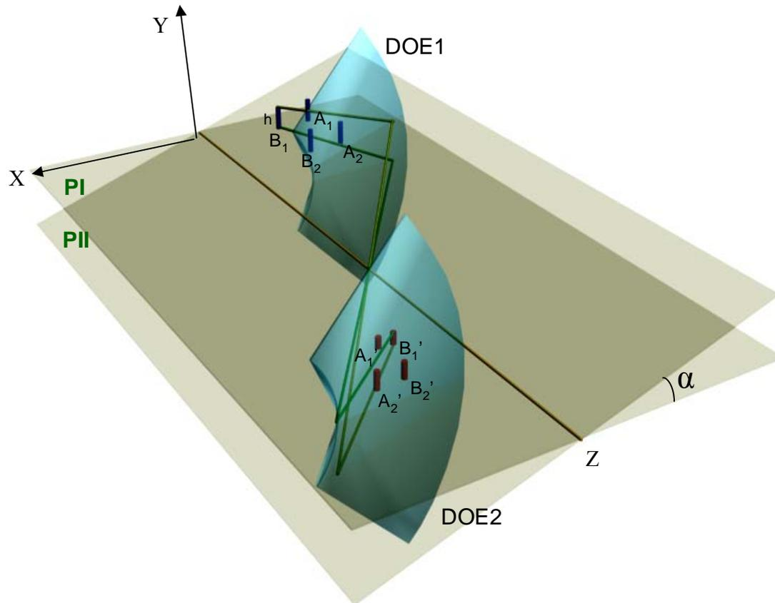
Figure 5.  $B_1'$  e  $B_2'$  are images of the objects  $B_1$  e  $B_2$  , all of them belonging to planes PI and PII.
