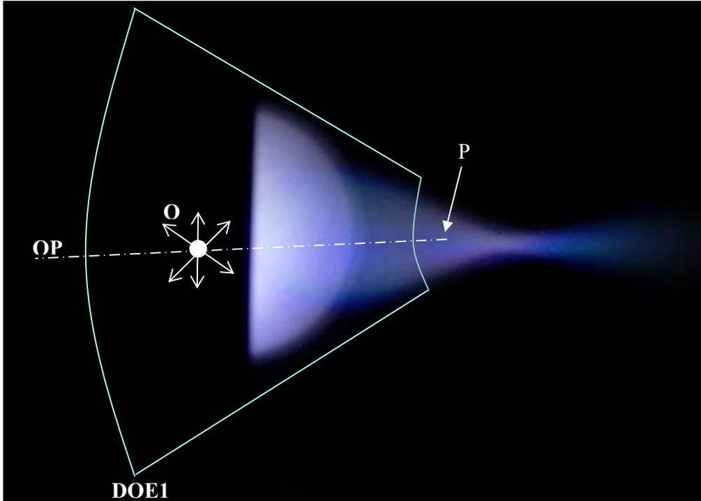
Figure 7. Light distribution reaching the pinhole P.
