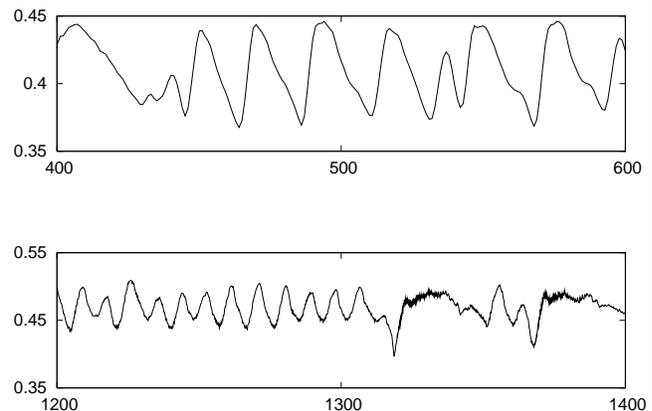
Fig. 6: Typical curves of the crack speed as a function of time during repetitive branching events for two different values of  $\beta$  (top: 8 and bottom: 4). One can see that the typical interval between maxima’s of the  $\beta = 8$  curve are approximately two times bigger than in the  $\beta = 4$  curve.
