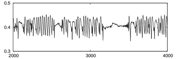
Fig. 4: Speed of the crack as a function of time. One can see the intermittent behavior of the crack speed. The burst of crack speed oscillation correspond to branching events while the regions where the speed is varying slowly correspond to a situation where the crack has divided into two branches that propagate together for a while before one of them takes over.  $\beta = 8$ .
