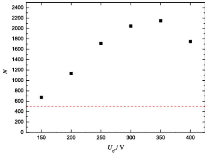
**Fig. 7** Number of ions,  $N$ , in the cavity mode volume versus rf-voltage,  $U_{rf}$ . The interval from 150 V to 400 V corresponds to ion densities between  $6.8 \times 10^8 - 1.1 \times 10^9 \text{ cm}^{-3}$ . The dashed line indicate the level above which the criterium for strong collective coupling is potentially satisfied.
