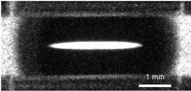
**Fig. 4** Image of a 3 mm long  $^{40}\text{Ca}^+$  Coulomb crystal with 88000 ions. The rf and end-voltages are 300 V and 1.7 V, respectively. The visible features outside the crystal region are from the trap and due to light scattered from the 397 nm beams as they pass through the mirrors. Due to the low magnification needed to image the whole crystal, no detailed crystal structure is visible.
