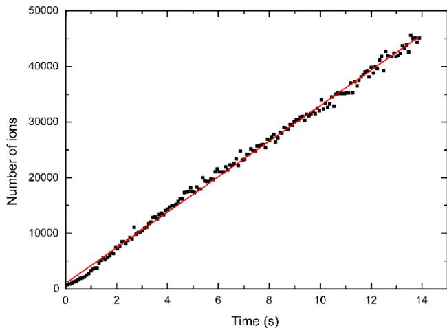
**Fig. 3** Number of ions loaded versus time when the ionization laser frequency is tuned close to the  $4s^2\ ^1S_0 \rightarrow 4s5p\ ^1P_1$  transition of  $^{40}\text{Ca}$ . The UV-power used for ionization was 20 mW and the oven temperature  $400^\circ\text{C}$ . The loading rate deduced from the linear fit is  $\sim 3200$  ions/s.
