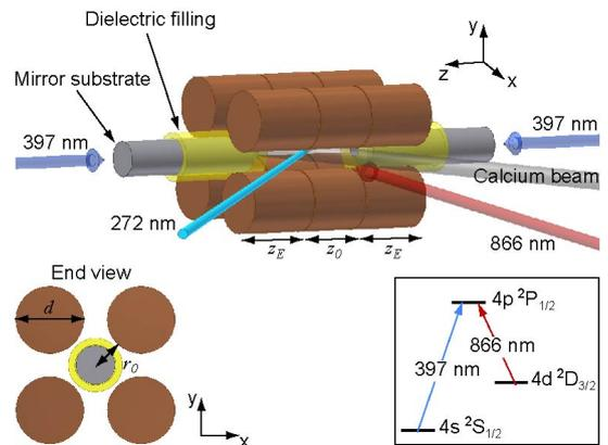
**Fig. 1** Schematic of the linear Paul trap with laser and atomic beams indicated. The dielectric fillings have been included to minimize the rf-fields along the trap axis ( $z$ -axis). The insert shows the level scheme used in Doppler laser cooling of  $\text{Ca}^+$ .
