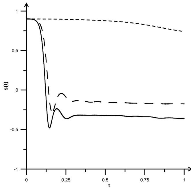
Figure 4: Spin polarization  $s$ , as a function of dimensionless time, for a cubic lattice, with  $\omega_0 = 2000$ ,  $\gamma = 10$ ,  $S = 10$ , and for different magnetic anisotropy values characterized by the anisotropy frequency  $\omega_D = 20$  (solid line),  $\omega_D = 50$  (long-dashed line),  $\omega_D = 100$  (short-dashed line).
