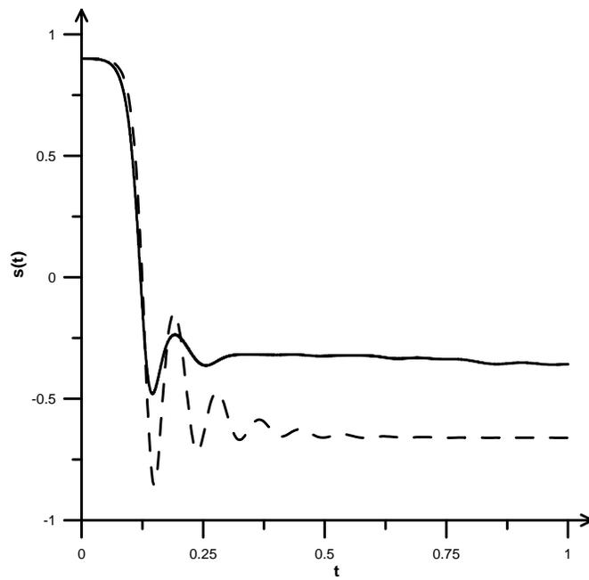
Figure 5: Spin polarization  $s$ , as a function of dimensionless time, for a cubic lattice, with  $\omega_0 = 2000$ ,  $\omega_D = 20$ ,  $\gamma = 10$ , and  $S = 10$ , for two different cases, when the dipole interactions are present (solid line) and when they are absent (dashed line).
