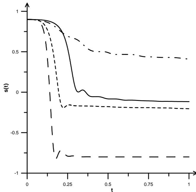
Figure 7: Difference in the behavior of spin relaxation for different sample shapes and orientations, under the same values  $\omega_0 = 2000$ ,  $\omega_D = 20$ ,  $\gamma = 30$ ,  $S = 10$ . The chain of spins along the  $z$ -axis (solid line); the chain of spins along the  $x$ -axis (long-dashed line); the plain of spins in the  $y - z$  plane (short-dashed line), and the plane of spins in the  $x - y$  plane (dashed-dotted line).
