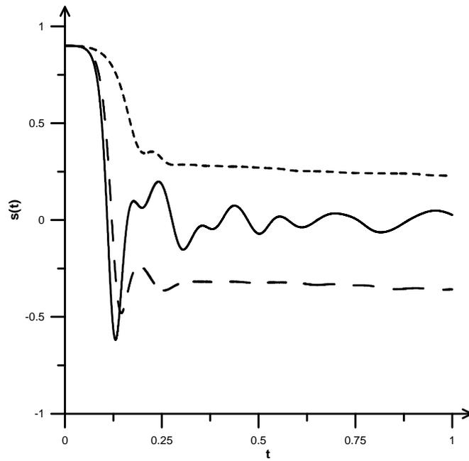
Figure 2: Reduced spin polarization  $s$ , as a function of dimensionless time, for a cubic lattice, with  $\omega_0 = 2000$  and  $\omega_D = 20$ , for the resonator damping  $\gamma = 1$  (solid line),  $\gamma = 10$  (long-dashed line), and  $\gamma = 50$  (short-dashed line). The sample of molecules with spin  $S = 10$  has the initial polarization  $s_0 = 0.9$ .
