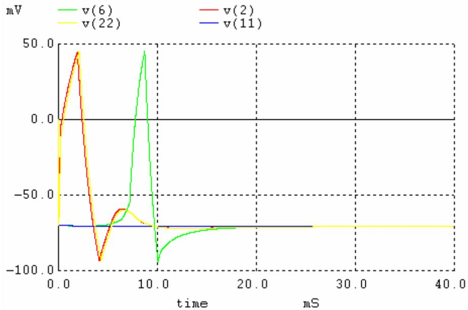
**Figure 13 A and C triggered but no output V(11); XOR because of capacitance reduction in segment 6.**
