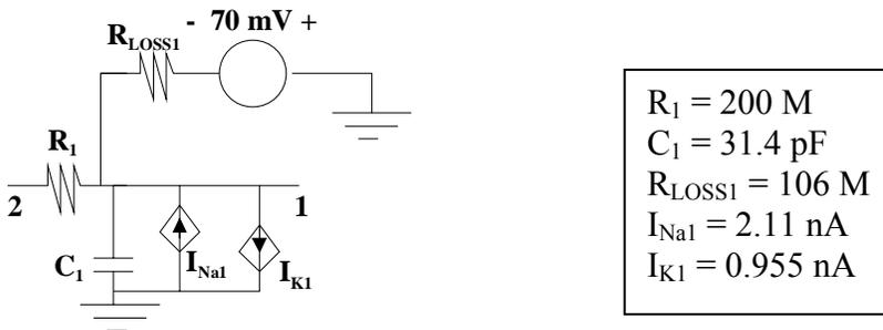
**Figure 5 Circuit model of a segment.**
