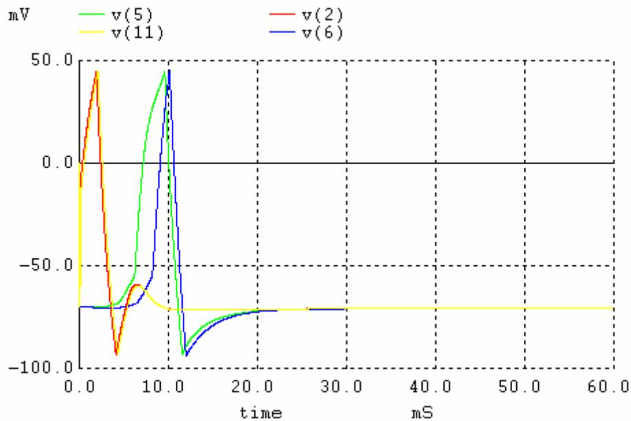
**Figure 9 Solitons injected at each end will collide and annihilate; no output V(11).**
