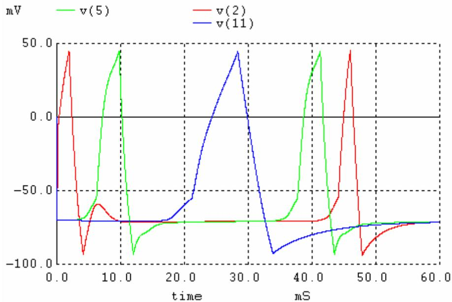
**Figure 8 Soliton that is reflected by a load capacitance of 60 pF.**
