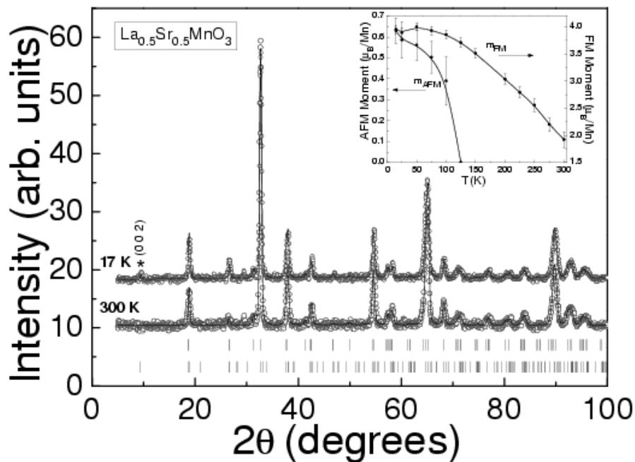
Figure: 8. Neutron diffraction pattern recorded on sample  $\text{La}_{0.5}\text{Sr}_{0.5}\text{MnO}_3$  at 17K and 300K. The symbol (\*) indicates the antiferromagnetic reflection. The inset shows temperature dependence of ferromagnetic and antiferromagnetic moment for  $\text{La}_{0.5}\text{Sr}_{0.5}\text{MnO}_3$ . The continuous lines are a guide for the eye.
