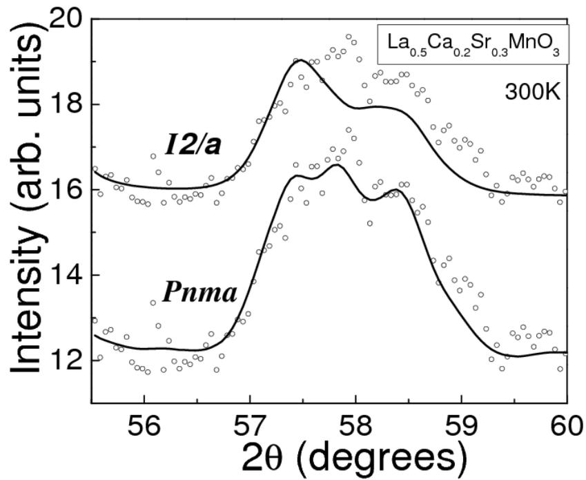
Figure: 1. A selected region (55.5 – 60°) of the fitted neutron powder diffraction patterns in two different space groups for  $\text{La}_{0.5}\text{Ca}_{0.2}\text{Sr}_{0.3}\text{MnO}_3$  sample at 300K. The observed data points are indicated with open circles while the calculated pattern is shown as a continuous line.
