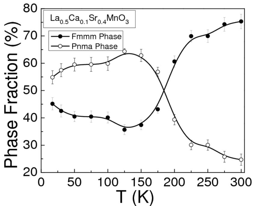
Figure: 2. Volume fraction of the *Fmmm* and *Pnma* phase with respect to temperature of the sample  $\text{La}_{0.5}\text{Ca}_{0.1}\text{Sr}_{0.4}\text{MnO}_3$  is shown. The continuous lines are a guide for the eye.
