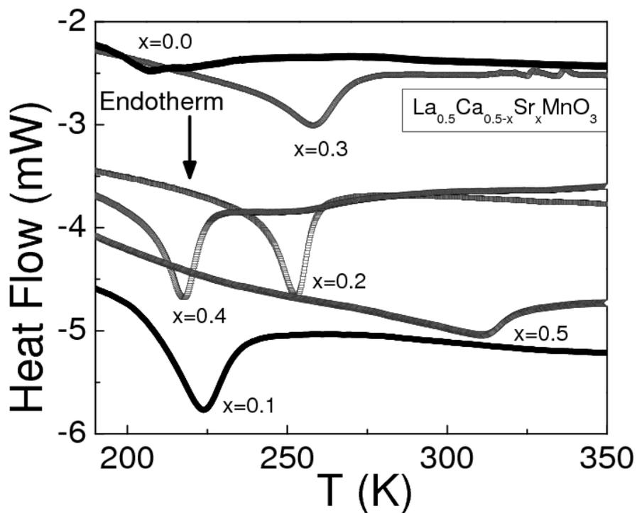
Figure: 9. The heat flow vs. temperature for  $\text{La}_{0.5}\text{Ca}_{0.5-x}\text{Sr}_x\text{MnO}_3$  ( $x = 0.2 - 0.5$ ) samples in the heating cycle.
