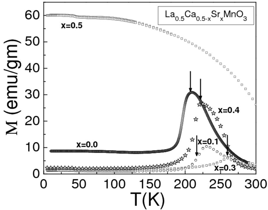
Figure: 4. The variation of magnetization with temperature in  $H = 1\text{T}$  for samples  $x = 0 - 0.5$ . For comparison the magnetization data for  $x = 0.0$  is taken from Ref. 7. The arrows in this figure show the endothermic peak transition temperature obtained from DSC.
