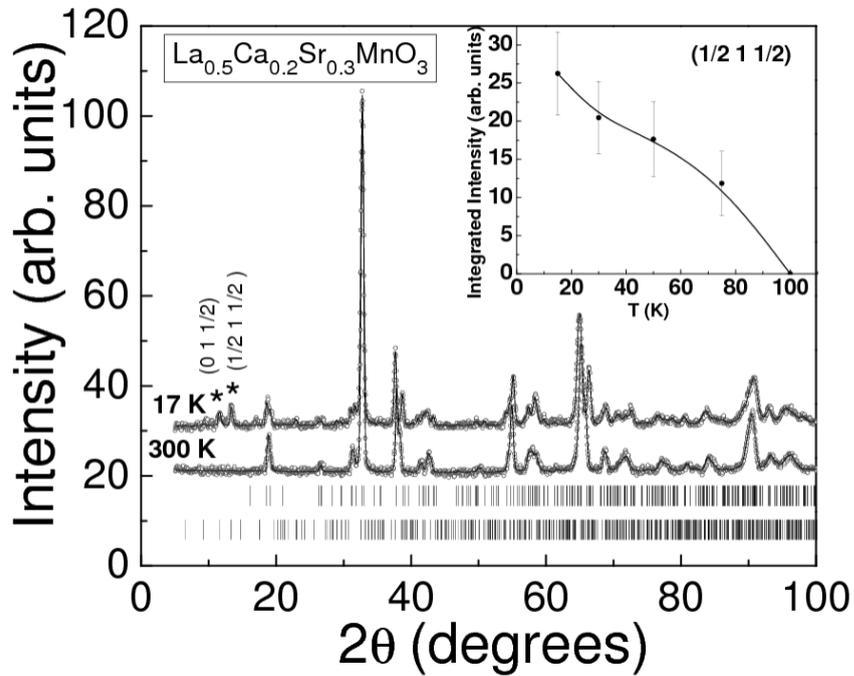
Figure: 6. Neutron diffraction pattern recorded on sample  $\text{La}_{0.5}\text{Ca}_{0.2}\text{Sr}_{0.3}\text{MnO}_3$  at 17K and 300K. The symbol (\*) indicates the AFM superlattice reflections. Continuous lines through the data points are the fitted lines to the chemical and magnetic structure described in the text. The inset shows the temperature variation of the antiferromagnetic superlattice reflection  $(\frac{1}{2}\ 1\ \frac{1}{2})$ . The continuous lines are a guide for the eye.
