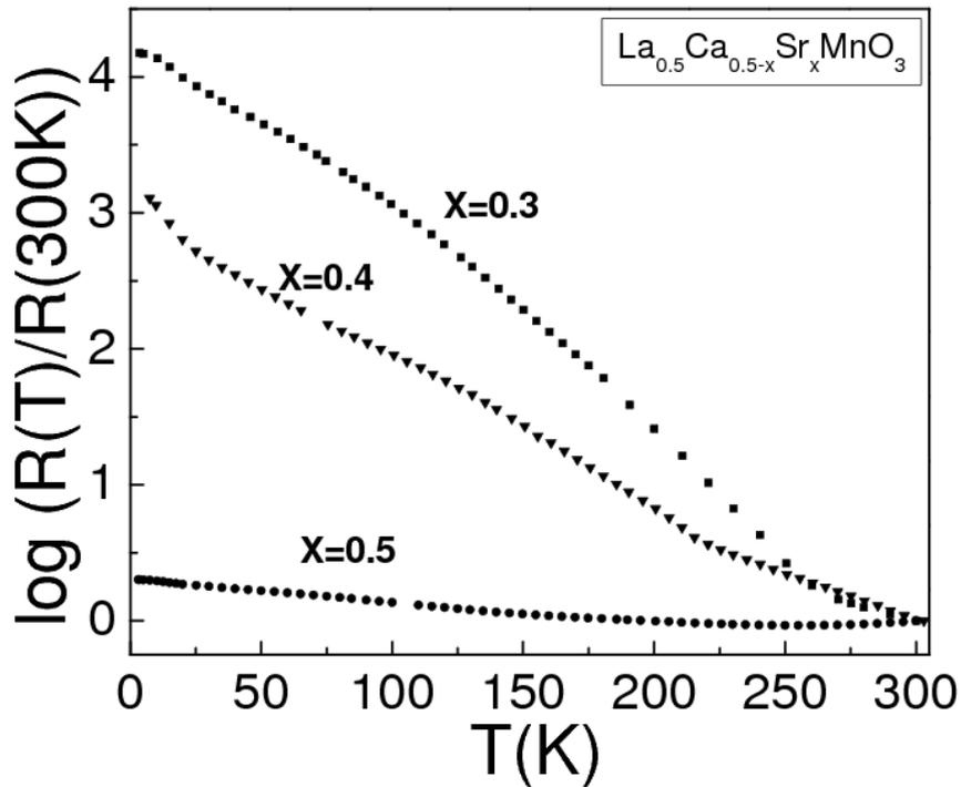
Figure: 5. The temperature dependence of normalized resistance for  $\text{La}_{0.5}\text{Ca}_{0.5-x}\text{Sr}_x\text{MnO}_3$  ( $x = 0.3, 0.4,$  and  $0.5$ ) samples.
