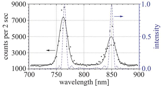
FIG. 4: Spectral distribution of down-conversion light with the central wavelengths of  $\lambda_1 = 762.8 \pm 0.4$  nm and  $\lambda_2 = 849.4 \pm 0.6$  nm, determined from a Gaussian fit (solid line). The lower peak number of counts at  $\lambda_2$  is due to a reduced efficiency of the spectrometer (with resolution 1.2 nm) towards infrared wavelengths. The dashed line shows the numerically simulated spectra obtained under the assumption of narrowband pumping.
