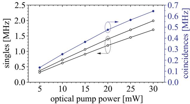
FIG. 3: Detected single and coincidence count rates depending on the pump power measured at the position of BBO crystals.
