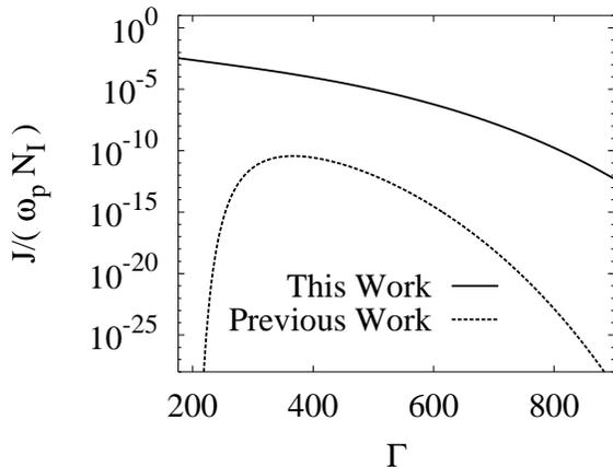
FIG. 1: Steady-state nucleation rate per ion as a function of  $\Gamma$ . “This Work” is the rate calculated from our model, and “Previous Work” is the rate calculated using the models of previous authors. Our calculations predict that the nucleation rate of a one-component plasma is  $> 10^5$  times higher than previously assumed for all values of  $\Gamma$ .
