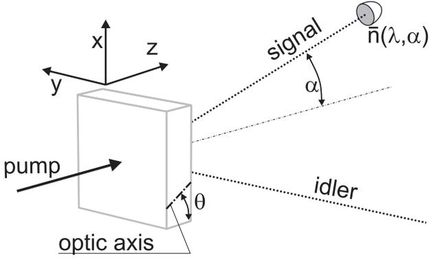
FIG. 1: Scheme of a measurement of the photon flux  $\bar{n}(\lambda, \alpha)$  of the spontaneous parametric fluorescence. The nonlinear crystal is pumped along  $z$ -axis. Out of the emerging parametric fluorescence we observe a small portion at the wavelength  $\lambda$  propagating at an angle  $\alpha$  to  $z$ -axis in the  $x$ - $z$  plane.
