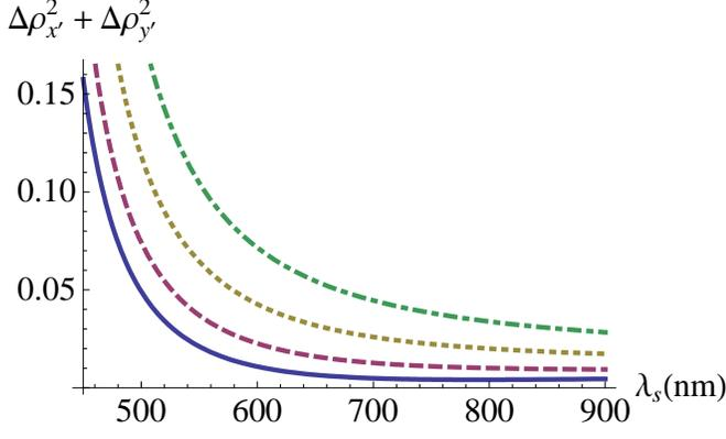
FIG. 4: (color online). Square idler spatial displacement coefficient  $\Delta\rho_x'^2 + \Delta\rho_y'^2$  in BBO for four different crystal cut angles  $\theta = 29^\circ$  (solid line),  $\theta = 31.3^\circ$  (dashed line),  $\theta = 35^\circ$  (dotted line) and  $\theta = 40^\circ$  (dot-dashed line).
