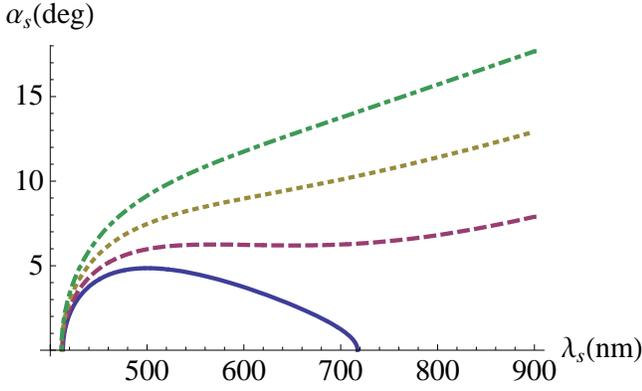
FIG. 3: (color online). Angle  $\alpha_s = \arcsin[ck^0(\omega)/\omega]$  at which perfectly phase-matched fluorescence at the wavelength  $\lambda = 2\pi c/\omega$  emerges outside the crystal. Plot corresponds to type-I phase-matching in BBO pumped at  $2\pi c/(2\omega_0) = 400$  nm for crystals cut at angles  $\theta = 29^\circ$  (solid line),  $31.3^\circ$  (dashed line),  $35^\circ$  (dotted line) and  $40^\circ$  (dash-dot line).
