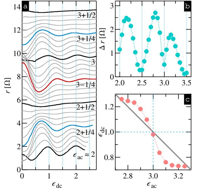
FIG. 2: (a) Differential resistance  $r$  vs  $\epsilon_{\text{dc}}$  at fixed  $\epsilon_{\text{ac}}$  from 2 to 3.5 in steps of 0.05. Traces are vertically offset in increments of  $0.4 \Omega$ . (b) Amplitude of the oscillations vs  $\epsilon_{\text{ac}}$ . (c) Position of the resistance maximum extracted from (a) near  $(\epsilon_{\text{ac}}, \epsilon_{\text{dc}}) = (3, 1)$ . Solid line corresponds to Eq. (1).
