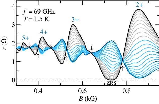
FIG. 1: (color online) Microwave magnetoresistance  $r$  under dc excitations, from  $I = 0 \mu\text{A}$  [black curve] to  $I = 22 \mu\text{A}$  [dark blue (dark grey) curve], in  $2 \mu\text{A}$  increments. Integers show the order of the MIRO peaks. The arrows mark zero-response nodes that largely remain immune to dc excitation.
