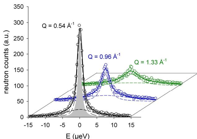
**Fig. 1** Incoherent quasielastic spectra of 8CB measured at  $T = 296$  K on the high resolution backscattering spectrometer IN16 (ILL – Grenoble). The resolution function of the apparatus is displayed as a filled gray shape. The solid lines are best fits of the data (see text.) using a two components model (dashed lines).
