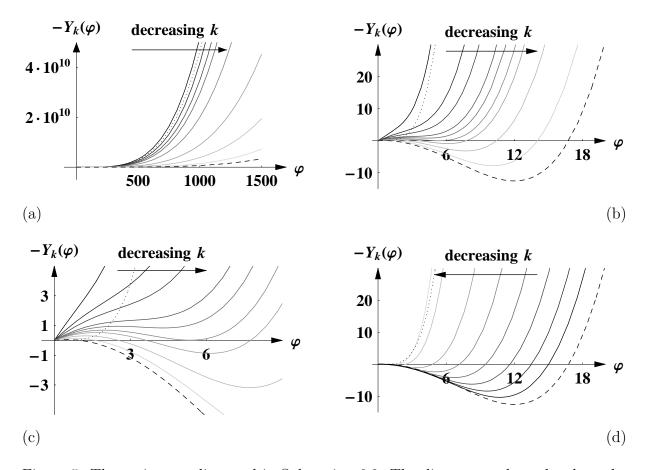
Figure 5: The trajectory discussed in Subsection 6.2. The diagrams a, b, and c show the potential for different values of k above  $k_{\rm T}$ , the diagram d for k-values below  $k_{\rm T}$ . The dotted (dashed) line is the fixed point (turning point) potential. The plots b and c are zooms into the diagram a at smaller  $\varphi$  values.
