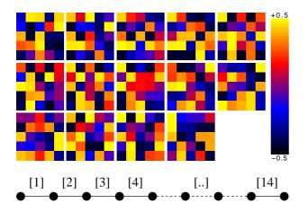
Fig. 7. Top: The receptive fields, Eq. (9), for the 14 winning coalitions [1], ..., [5] (first row) [6], ..., [10] (second row) and [11], ..., [14] (third row) as a function of the  $5 \times 5$  input field, compare Fig. 5. For the response of the 14 winning coalitions with respect to the ten reference input patterns compare Fig. 6. Note that the receptive fields can be both positive as well as negative, see the color-coding.
