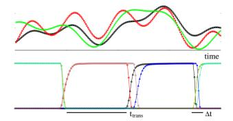
Fig. 1. Schematic illustration of general or fluctuating activity patterns (top) and of transient-state dynamics (bottom), which is characterized by typical time scales  $t_{trans}$  and  $\Delta t$  for the length of activity-plateau and of the transient period respectively.
