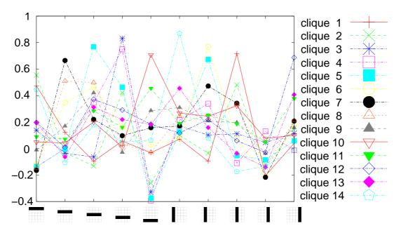
Fig. 6. The response, as defined by Eq. (8), for the 14 winning coalitions in the dHAN layer (compare Fig. 7) to the ten reference patterns, viz the 5 horizontal bars and the 5 vertical bars of the  $5 \times 5$  input field.
