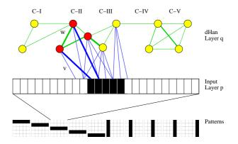
Fig. 4. Schematic representation of the information flow from a raw pattern (bottom) via the input layer (middle) to the dHan layer (top). The synaptic strength  $v_{ij}^{pq}$  connecting the input with the dHan layer (denote 'v' in the graph) are adapted during the learning process (illustrated selectively by respective thick/thin blue lines in the graph).
