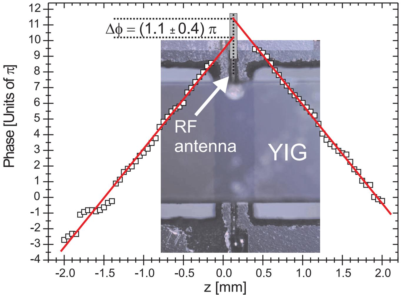
FIG. 2: (Color online) Phase accumulation for BVMSW geometry. The measured excitation phase is  $(1.1 \pm 0.4)\pi$ . The applied bias magnetic field is 1835 Oe. Spin wave carrier frequency and wavevector are 7.132 GHz and  $(-198 \pm 1) \text{ cm}^{-1}$  respectively. The inset shows a micrograph of the used structure.
