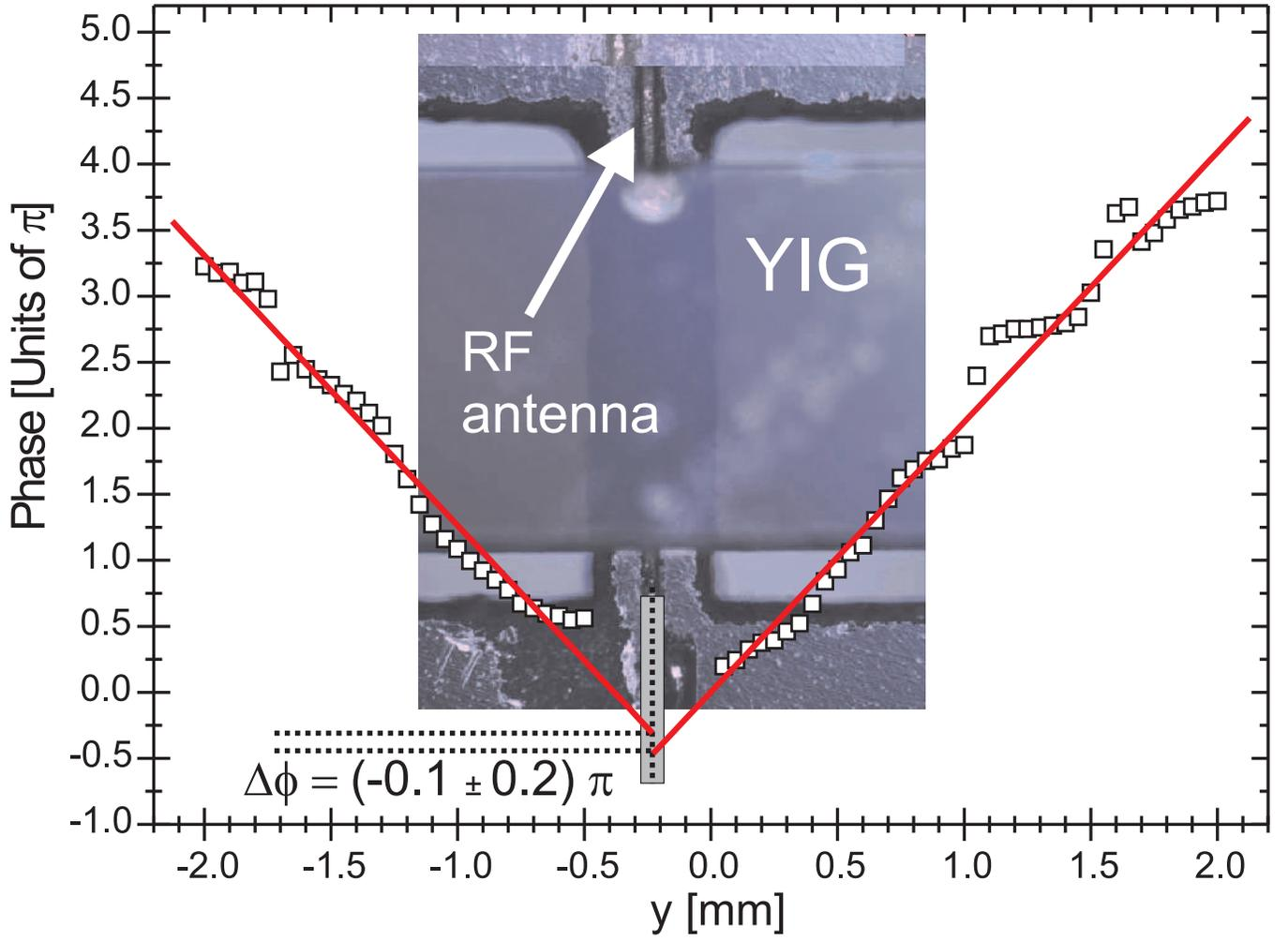
FIG. 3: (Color online) Phase accumulation for MSSW geometry. The measured excitation phase is  $(-0.1 \pm 0.2)\pi$ . The applied bias magnetic field is 1825 Oe. Spin wave carrier frequency and wavevector are 7.132 GHz and  $(64.21 \pm 0.04) \text{ cm}^{-1}$  respectively. The inset shows a micrograph of the used structure.
