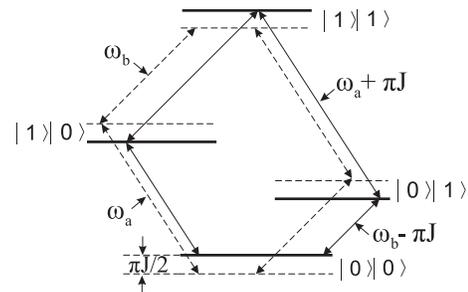
FIG. 2: Energy level diagram for (solid lines) two spins coupled by a Hamiltonian of the form of  $2\pi\hbar J I_z^a I_z^b$  and (dashed lines) two uncoupled spins.
