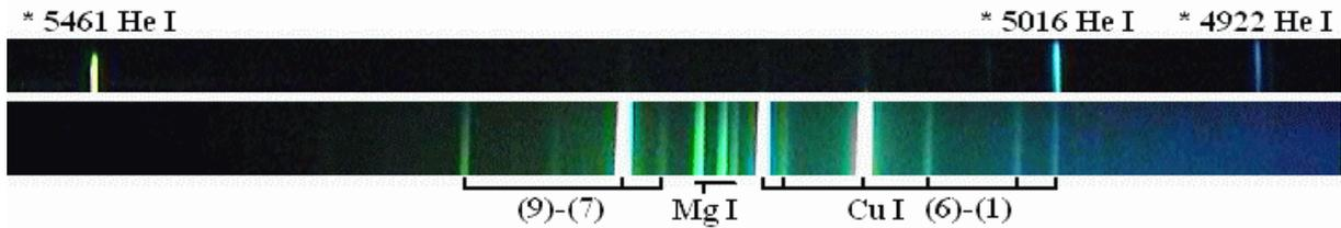
**Fig.6. HVEWD spectrum at the blue-green range, 20 ms after the discharge ignition.**
