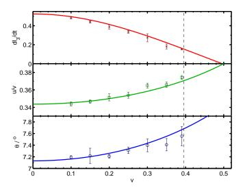
FIG. 15: The measured physical bridge half-length growth rate  $dl_3/dt$ , bridge speed u and bridge orientation  $\theta$  from type B collisions with  $\alpha=20^{\circ}$ , compared to CKS predictions. The simulation had  $\Delta x=0.5$  and were of sufficient size that signals emitted from the box centre at t=0 would reach the corners of the yz-plane by  $t=60\eta^{-1}$  (except for v=0.39 when this value was  $120\eta^{-1}$ ).
