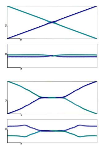
FIG. 4: Isosurfaces of  $|\phi|=0.5\eta$  and  $|\psi|=0.5\nu$  from a type A collision: (1,0)+(0,1). The upper two frames are from  $t=-6\eta^{-1}$ , showing the attraction of the strings towards each other and intersection at negative times rather than the Nambu-Goto value of t=0. The lower two frames are from the later time of  $t=+30\eta^{-1}$ , showing the established bridge and Y-junctions. The initial speeds were v=0.2 and the strings made an angle  $\alpha=20^{\circ}$  to the z-axis.
