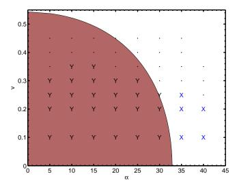
FIG. 6: Incident velocities v and angles  $\alpha$  which are seen in simulations to yield Y-junctions when  $\mu_1 = \mu_2$  (i.e. S = 0) and R = 0.840. Here Y denotes the formation of a bridge with Y-junctions at either side, points that the strings passed through each other and X denotes that the strings became locked together to form an X-junction. The CKS prediction is that the region beneath the curve could yield Y-junctions.
