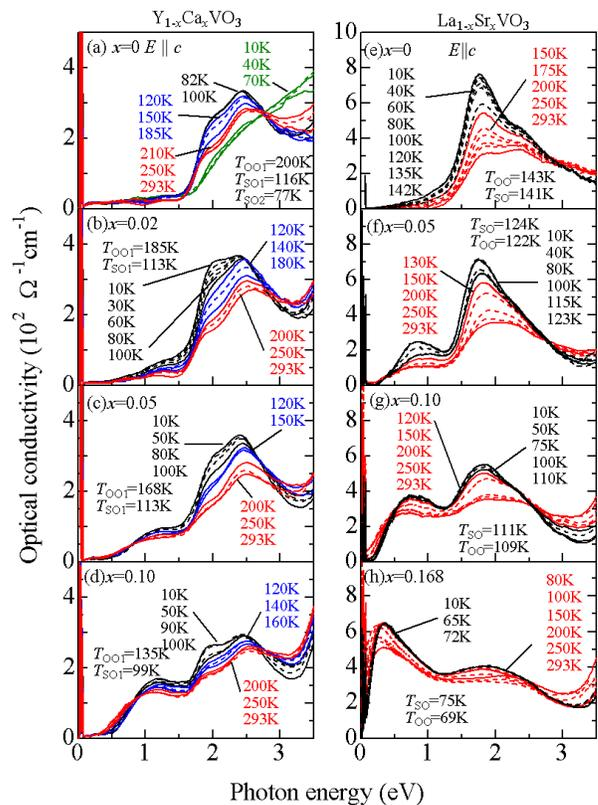
FIG. 4: (Color online) Left panel: The temperature dependence of the optical conductivity spectra for  $\text{Y}_{1-x}\text{Ca}_x\text{VO}_3$  with (a)  $x = 0$ , (b) 0.02, (c) 0.05, and (d) 0.10, respectively. Right panel: The temperature dependence of the optical conductivity spectra for  $E \parallel c$  in  $\text{La}_{1-x}\text{Sr}_x\text{VO}_3$  with (e)  $x = 0$ , (f) 0.05, (g) 0.10, and (h) 0.168, respectively.
