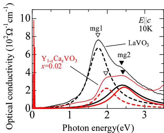
FIG. 6: (Color online) Optical conductivity spectra at 10K for  $E||c$  in  $\text{Y}_{1-x}\text{Ca}_x\text{VO}_3$  with  $x = 0.02$  and  $\text{LaVO}_3$ , respectively. The thick dashed and solid lines represent the Lorentz oscillators assumed for the fitting of the two-components of the Mott-gap excitation,  $mg1$  and  $mg2$ , respectively.
