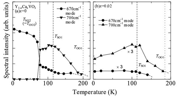
FIG. 8: (Color online) Temperature dependence of the spectral intensity of the phonon peaks around  $670cm^{-1}$  (closed circle) and  $700cm^{-1}$  (closed triangle) in  $Y_{1-x}Ca_xVO_3$  with (a)  $x = 0$  and (b)  $x = 0.02$ , respectively. The dash-dotted, dashed, and dotted lines indicate  $T_{SO2}$  ( $=T_{OO2}$ ),  $T_{SO1}$ , and  $T_{OO1}$ , respectively.
