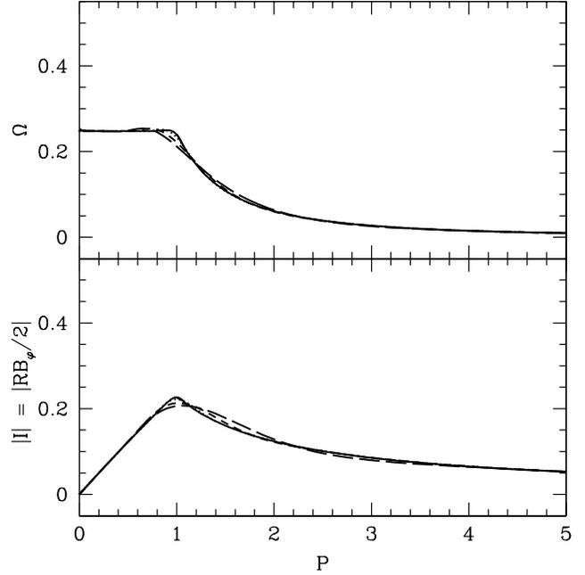
**Figure 6.** Transverse variations of the field-line invariants,  $\Omega$  and  $|I|$ , for model A as a function of the magnetic field stream function  $P$ . In each panel four curves are shown: the star-disk surface (solid line),  $r = 10^2$  (dotted),  $r = 10^4$  (short-dashed), and  $r = 10^6$  (long-dashed). Over a range of six orders of magnitude in distance, the values of  $\Omega$  and  $|I|$  are conserved to better than 12%.
