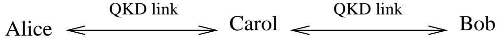
FIG. 3: QKD bridge: Alice and Bob are out of the QKD range, they want to use Carol as a bridge to communicate securely the shared key.
