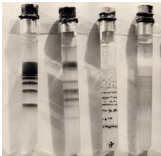
Fig. 1. (colour online) Experimental examples of Liesegang patterns in test tubes. Agent A is injected from the open end (top) of the tube, which contains agent B dissolved in a gel, yielding a linear geometry (Figure by D. B. Siano, http://commons.wikimedia.org/wiki/Image:Liesegangrings.jpg ).
