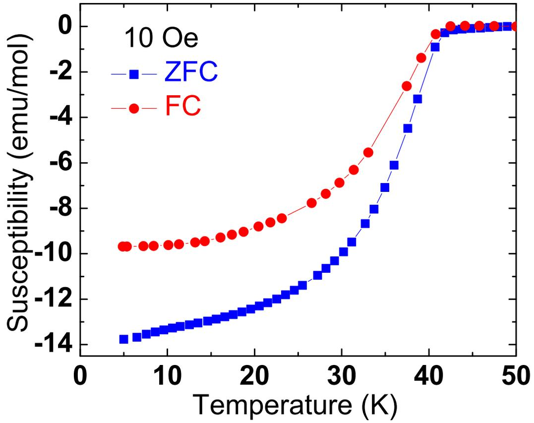
FIG. 3: Temperature dependence of magnetic susceptibility as a function of temperature for the sample annealed at 1160 °C in the zero-field cooled (ZFC) and field-cooled measurements at 10 Oe.
