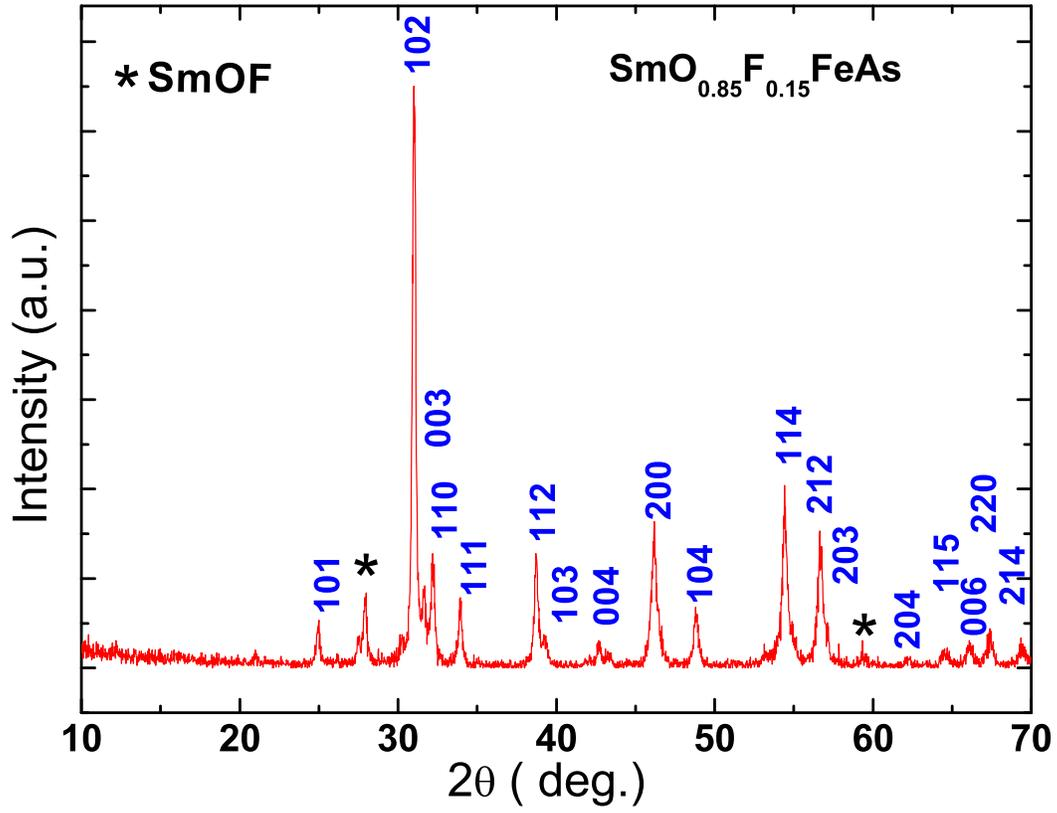
FIG. 2: X-ray diffraction pattern for the sample with nominal composition  $SmFeAsO_{1-x}F_x$  ( $x=0.15$ ) annealed at  $1160\text{ }^\circ\text{C}$ . A tiny impurity phase SmOF is observed.
