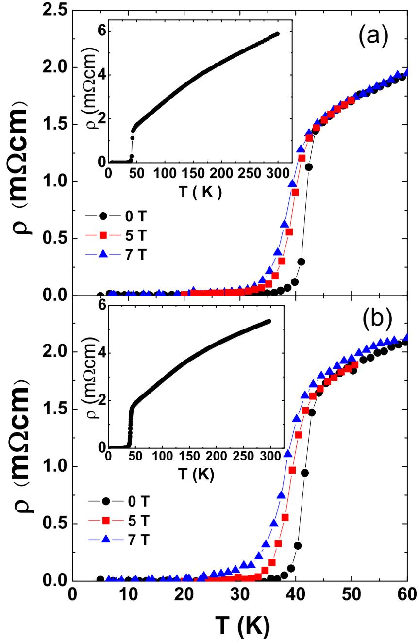
FIG. 4: Temperature dependence of resistivity without magnetic field and under magnetic field of 5 and 7 T for the samples annealed at 1160 °C (a) and 1200 °C (b), respectively. Inset shows the resistivity from 300 K to 5 K.
