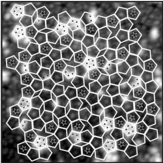
FIG. 4: The five-fold surface of *i*-Al-Pd-Mn with a Bi coverage of 0.13 ML as in Fig. 1(a). A Penrose P1 tiling edge length 7.8 Å has been superimposed. Bismuth atoms only decorate ‘top’ pentagonal tiles and many of the ‘bottom’ pentagonal tiles enclose a five-fold depression (‘dark star’). These are indicated with a star motif.
