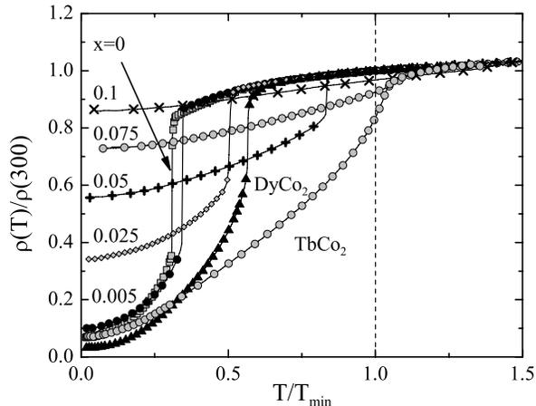
FIG. 6: Normalized resistivity  $\rho(T)/\rho(300)$  against normalized temperature  $T/T_{\min}$  for  $\text{Ho}(\text{Co}_{1-x}\text{Al}_x)_2$  alloys and  $\text{DyCo}_2$ ,  $\text{TbCo}_2$  compounds<sup>39</sup>.
