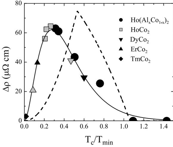
FIG. 9: The resistivity drop  $\Delta\rho$  at Curie temperature of  $\text{Ho}(\text{Co}_{1-x}\text{Al}_x)_2$  alloys and of some  $R\text{Co}_2$  compounds<sup>39,44</sup>. Broken line is theoretical  $\Delta\rho$ , scaled with  $\rho(T_m)=100 \mu\Omega \text{ cm}$ . The gray symbols stand for data under pressure for corresponding compounds<sup>43</sup>.
