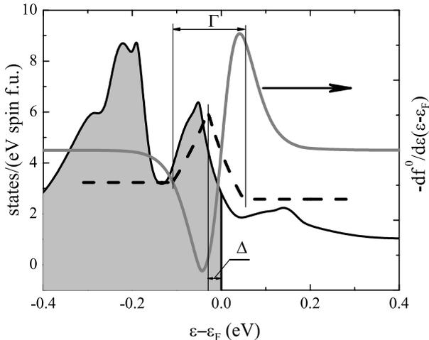
FIG. 3: DOS of  $R\text{Co}_2$  compounds in a vicinity of the Fermi level (solid line)<sup>20</sup>. The gray line shows  $-df^0/d\varepsilon(\varepsilon - \varepsilon_F)$  at  $T=300$  K ( $f^0$  is Fermi distribution function) to indicate the energy region important for transport properties. The broken line is the model state density, used for thermopower calculations.  $\Gamma$  is the width of the model DOS peak,  $\Delta$  - is the distance from Fermi level to the center of the peak.
