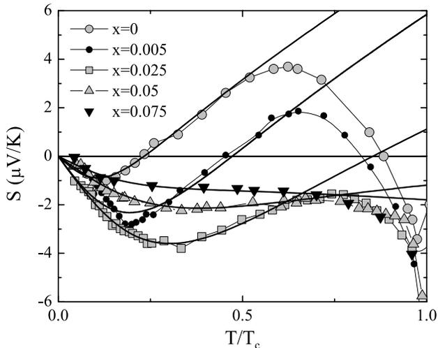
FIG. 12: Low temperature thermopower of  $\text{Ho}(\text{Co}_{1-x}\text{Al}_x)_2$ . The solid lines represent the Nordheim-Gorter expression (8) with parameters, listed in Table I.
