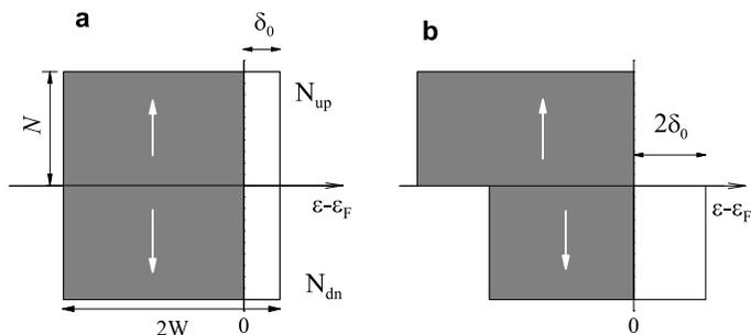
FIG. 7: The model of  $3d$  DOS: **a.** Non polarized state at  $T=0$  K; **b.** Polarized state at  $T=0$  K.  $2W$  is the  $3d$  band width,  $\delta_0$  is the distance from Fermi energy to the top of  $3d$  band and  $N$  – DOS magnitude.
