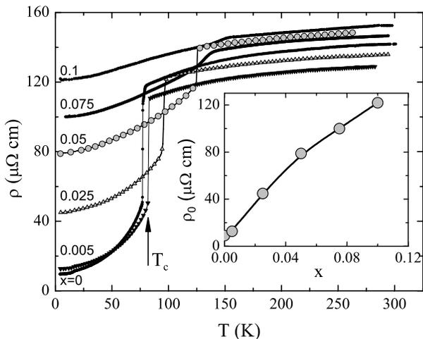
FIG. 1: Temperature dependent resistivity of  $\text{Ho}(\text{Co}_{1-x}\text{Al}_x)_2$  for various Al concentrations. The inset shows the composition dependence of the residual resistivity, measured at 4.2 K.
