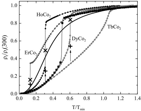
FIG. 10: Normalized resistivity of  $R\text{Co}_2$  compounds<sup>39</sup> and  $\text{Ho}(\text{Co}_{0.975}\text{Al}_{0.025})_2$  alloy (■). The solid line is the resistivity of  $\text{YCo}_2$ .  $\rho_t = \rho(T) - \rho(4.2)$ . 'X' and '+' indicate resistivity at  $T_c$ , including corrections for  $\rho_{\text{spd}}$  and  $\rho_{\text{sw}}$  in paramagnetic and ferrimagnetic phase, respectively.
