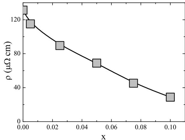
FIG. 5: Temperature – induced part of resistivity ( $\rho(250) - \rho(4.2)$ ) of  $\text{Ho}(\text{Co}_{1-x}\text{Al}_x)_2$  alloys.
