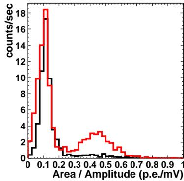
Fig. 7. *area/amplitude* (p.e./mV) distribution for  $^{57}\text{Co}$  source data (red) and BG data (black). The peaks at *area/amplitude*  $\sim 0.1$  and  $\sim 0.45$  are due to PMT dark noise and scintillation signals, respectively.
