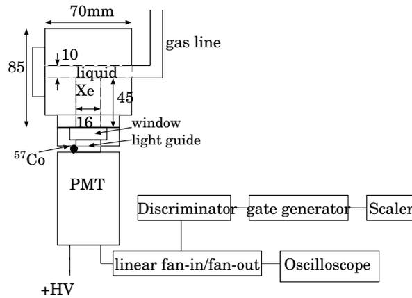
Fig. 2. Cross section of the liquid xenon vessel and measurement diagram; the inner volume of the high pressure vessel is 15 cc. The  $^{57}\text{Co}$  source is located at edge of light guide.
