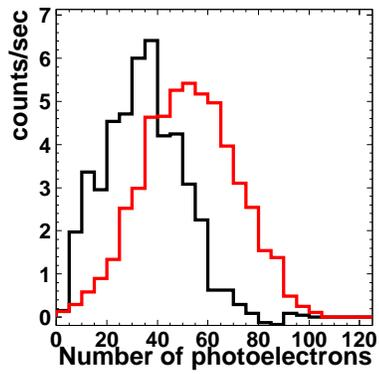
Fig. 9. p.e. distribution at ( $T=1\text{ }^{\circ}\text{C}$ ,  $P=5.5\text{ MPa}$ ). The black line shows the data. The red line shows the MC.
