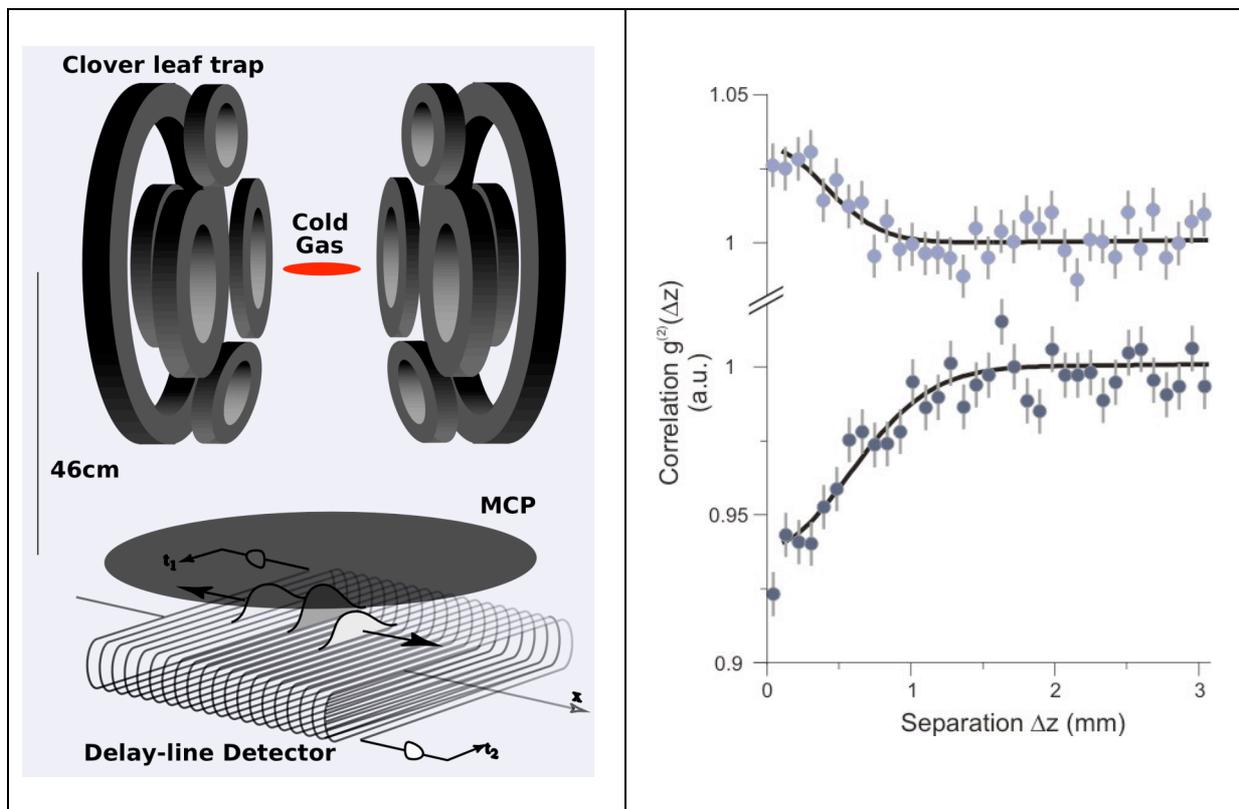
Figure 2. Experimental setup at the Institut d'Optique. The atoms are held in a magnetic trap where laser and evaporative cooling produce a cloud of  $10^5$  atoms at a temperature of order one microKelvin. The detector is 80 mm in diameter and uses a system of delay line anodes to achieve a spatial resolution of about 0.5 mm.
