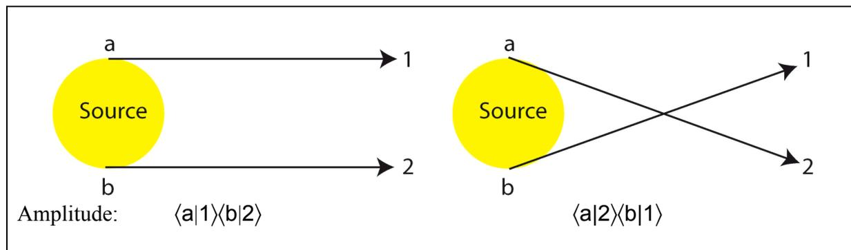
Box 2. Quantum interpretation of intensity correlations. Two photons from two source points,  $a$  and  $b$  are detected at points 1 and 2 following the two possible pairs of paths shown above. Each pair of paths corresponds to a quantum amplitude, and these amplitudes are added to find the probability to detect 2 photons:
