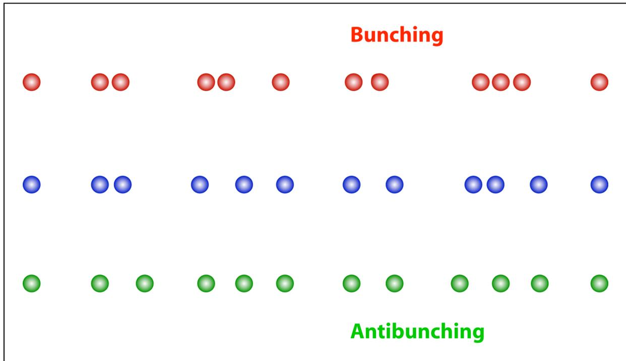
Box 3. The figure above illustrates the meaning of the terms bunching and antibunching. Suppose the spheres in each row represent the positions of a group of particles along a line. (They could also represent the arrival times at a detector.)
