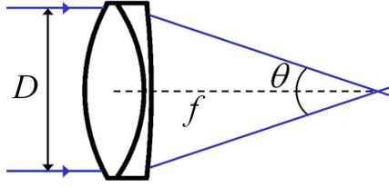
Fig. 1. Two parallel beams separated by a distance  $D$ , produce an optical lattice at the focal plane of the lens. We use an achromatic doublet lens to minimize the aberration of the off-axis beams. The highly curved surface faces the incident parallel beams.
