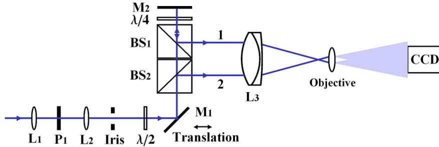
Fig. 2. Experimental set-up for creating and imaging the optical lattices with real-time control of periodicity.  $L_1$ ,  $L_2$  are singlet lenses;  $P_1$  is a pinhole;  $M_1$  and  $M_2$  are mirrors;  $BS_1$  and  $BS_2$  are polarizing cube beam splitters; and  $L_3$  is an achromatic doublet lens.
