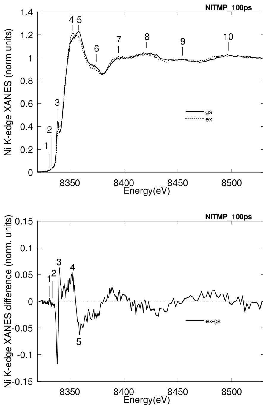
**Fig. 1 Upper frame: Experimental Ni K-edge XANES spectrum of Ni(II)-TMP, ground state,  $S_0$  (solid line), and of its 100ps laser photoproduct, containing 45-50% of an excited triplet  $T_1$  state. Lower frame: XANES difference spectrum of data reported in the upper frame.**
