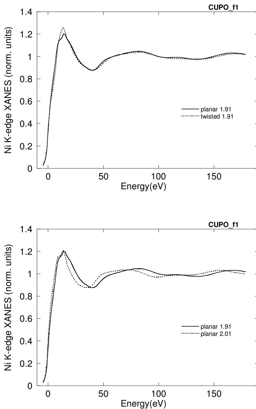
Fig. 6. Upper frame: Theoretical XANES spectra of structure A (planar, solid line) and structure B (twisted line), having the same  $d(\text{Ni-N}_p)$  distance. Lower frame: Theoretical XANES spectra of structure A with two different  $d(\text{Ni-N}_p)$  distances. Distance values are reported in the legend.
