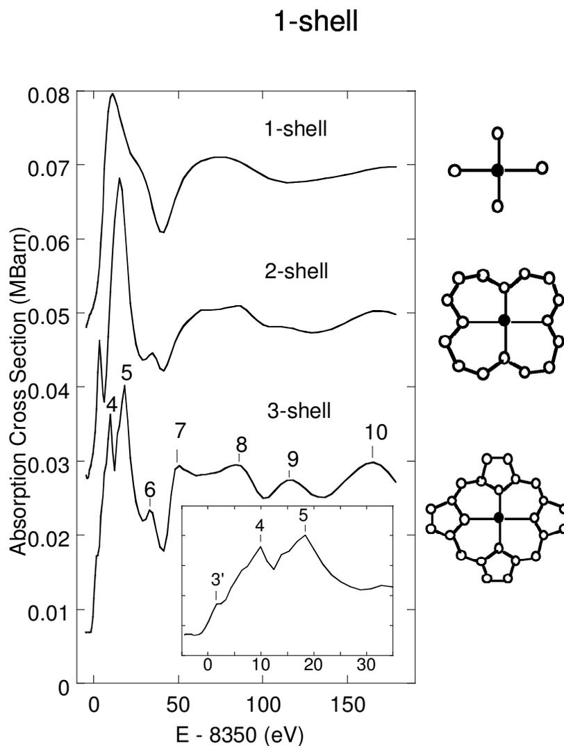
Fig. 2. Theoretical XANES spectrum of square planar Ni(II)-porphyrin as a function of the cluster size. Calculations are done without any damping coming from inelastic losses to emphasize the origin of each feature. According to this set of calculations, peaks 4 and 5 (absent in 1-shell and 2-shell calculations) can be attributed to MS signal coming from electron pathways extending all over the 3-shell cluster.
