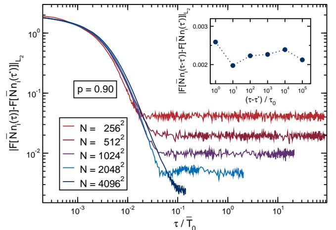
FIG. 4: (Color online)  $L_2$  norm of the difference between the distribution function  $F[n_i(\tau)]$  at time  $\tau$  and the quasi-stationary distribution  $F[n_i(\tau^*)]$  for different system sizes. The inset shows the dependency of this quantity on the time difference for the  $N = 4096^2$  system in the quasi-stationary regime. Note the different axis scales.
