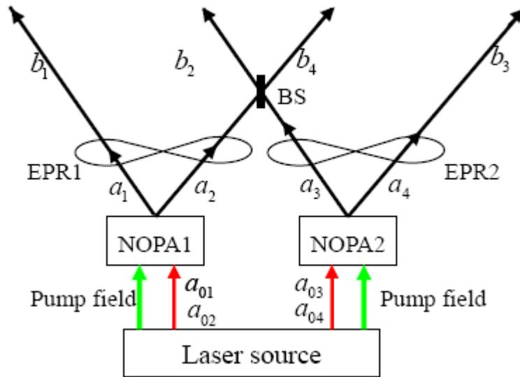
Fig.1 Principle schematic for CV quadripartite TTPC generation
