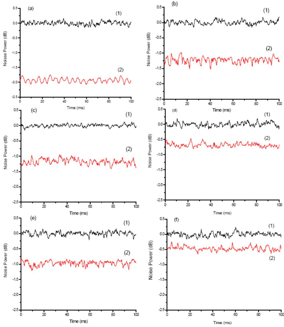
Fig.3 The measured correlation variances of the TTPC at 2 MHz
