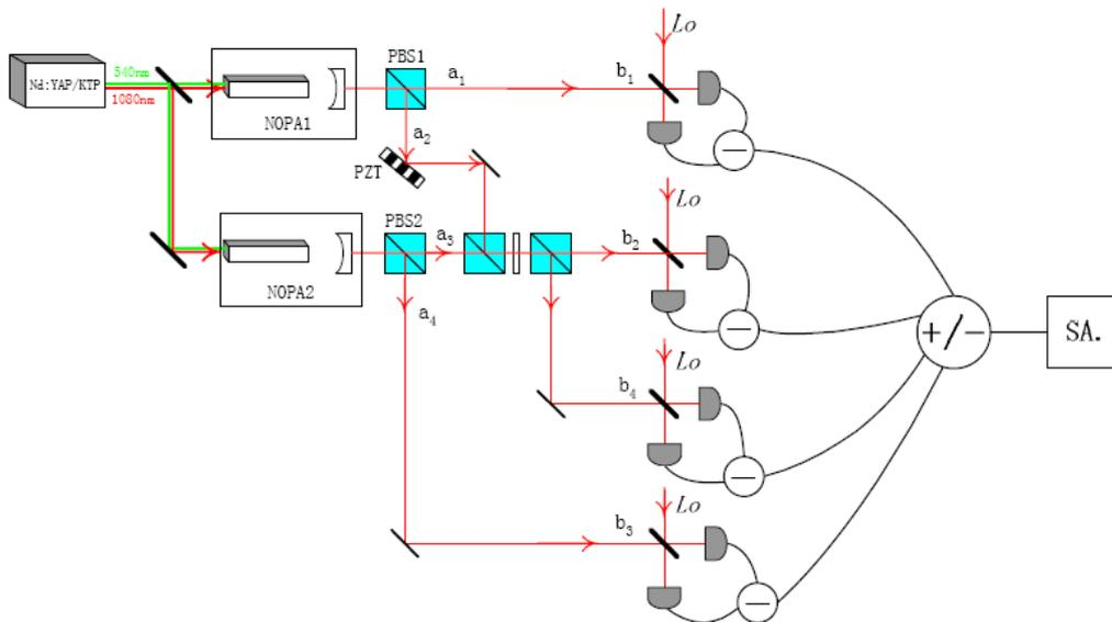
Fig.2 Schematic of the experimental setup for the TTPC generation
